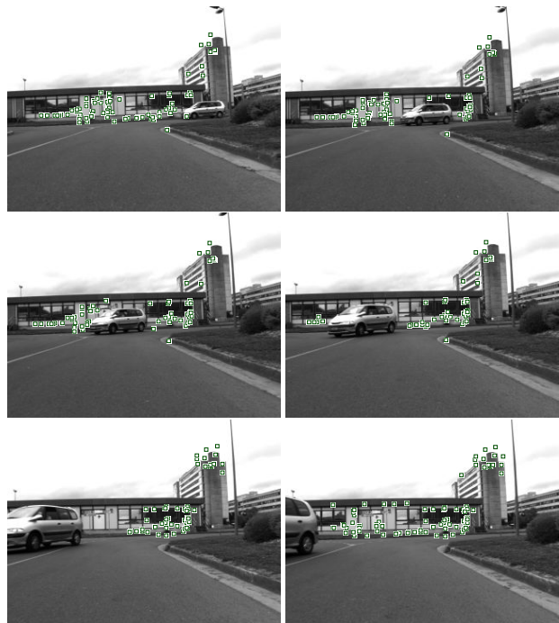
Figure 13. Sequence of images obtained during the execution of a navigation experiment. The points used for navigation re-appear after being occluded and disoccluded by a moving car.
