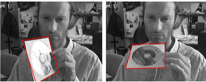
Fig. 8. Robust visual tracking of a planar target with the ESM algorithm. The output of the algorithm is a homography matrix.
