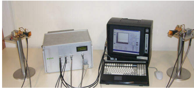
Fig. 1 Channel sounder at 60 GHz realized by IETR
