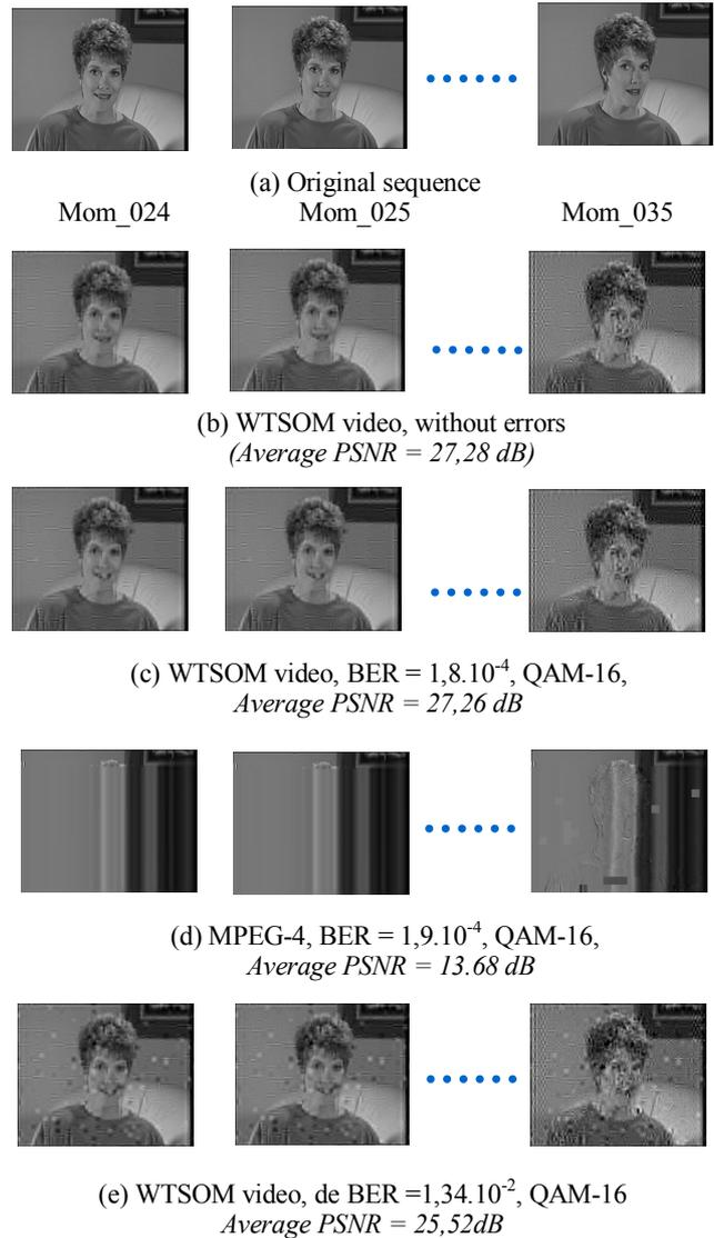
Figure 6. Sequence transmitted through ideal and AWGN channel comparable compression rate : (a) original sequence (b) WTSOM video, without errors, (c) WTSOM video,  $BER = 1,8.10^{-4}$ , (d) MPEG-4,  $BER = 1,9.10^{-4}$  (e) WTSOM video,  $BER = 1,32.10^{-2}$
