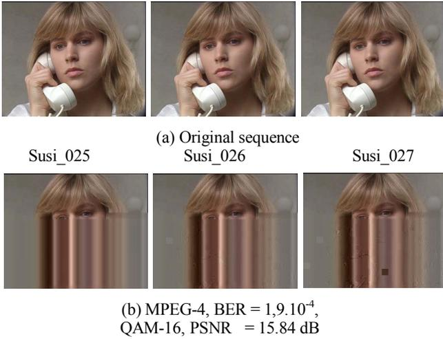
Figure 1. Transmission through ideal channel (without errors) and through AWGN channel:
