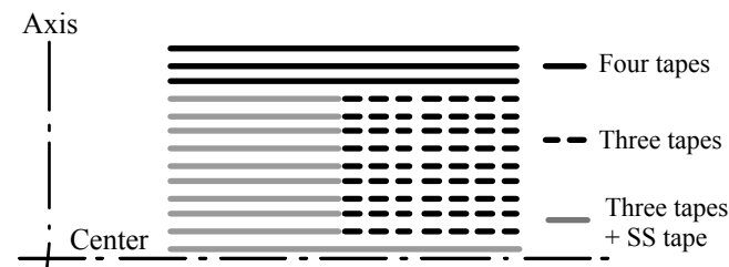
Fig. 3. Conductor distribution within half of the coil.
