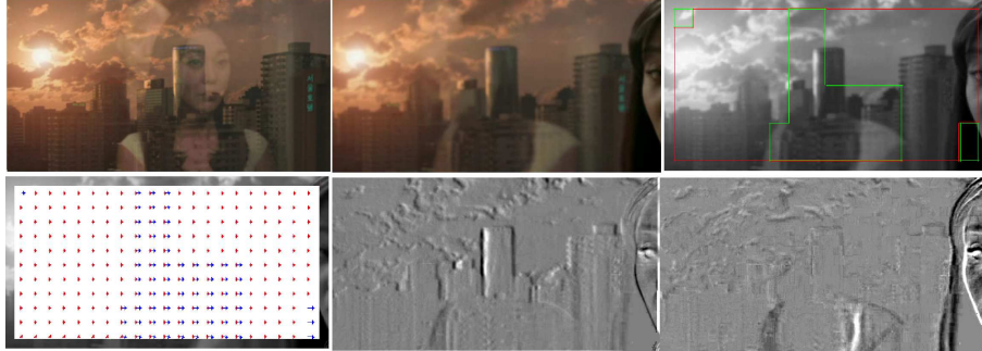
Figure 10: Example of a movie depicting two people reflected on an apartment window. From left to right and top to bottom: the first frame of the sequence; one of the three images corresponding to the reported results later in the sequence; the obtained segmentation into the transparent layer supports (the green polygonal line in the middle roughly encloses the reflected people); the velocity fields supplied by the estimated affine motion models; displaced frame differences computed by compensating the motion of one of the two layers.
