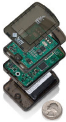
Figure 13. Sun SPOT wireless sensor, sensor board on top, processor and radio in the middle and battery board on the bottom
