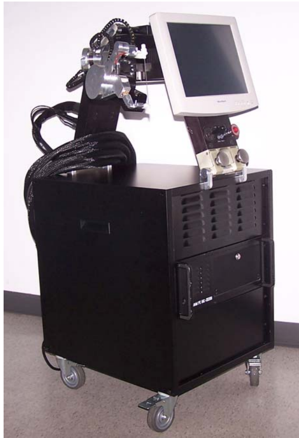
Figure 2: Revolving Needle Driver on the AcuBot robot
