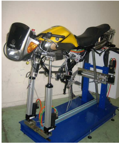
Fig. 6. Constructed riding motorcycle simulator
