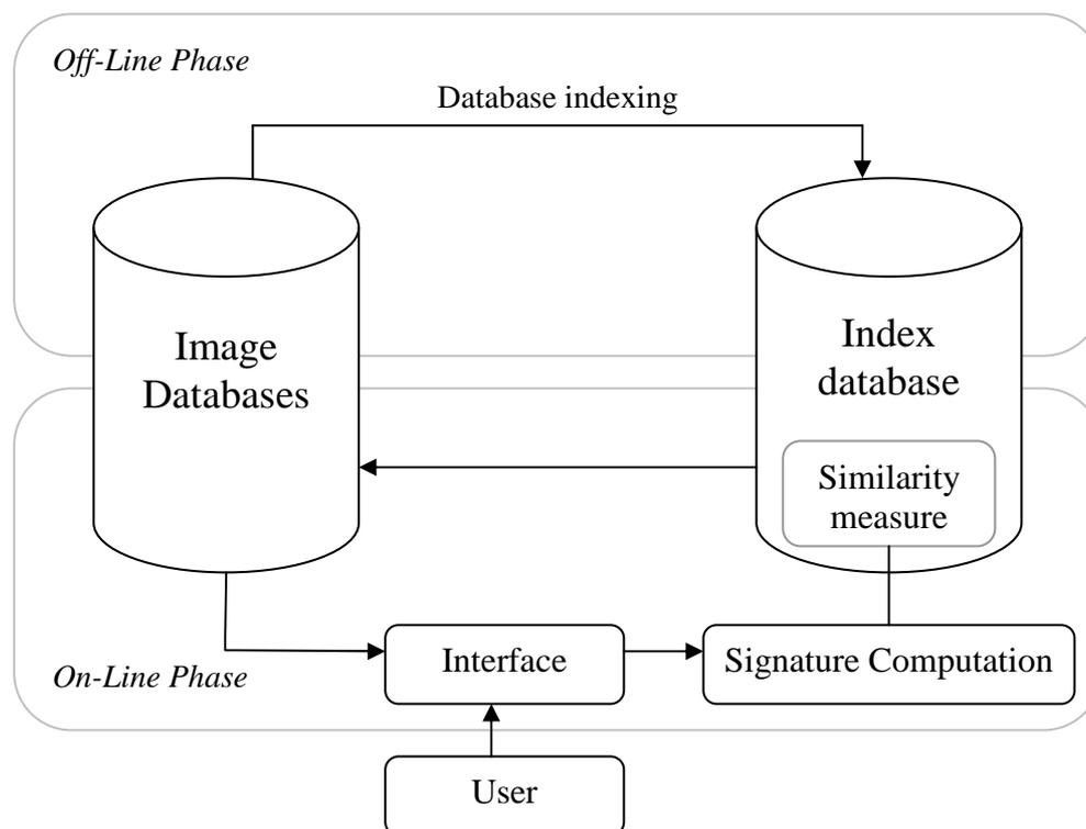
**Figure 2.** Content based image retrieval architecture
