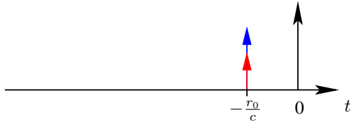
Fig. 6. Time reversed signals (Fig. 5) after propagation from each receiver to the target: pulses arrive simultaneously on the right space point, resulting to focusing.
