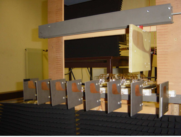
Fig. 1. The SIMIS radar, consisting of one emitting antenna (top right) and an eight-element receiving array.
