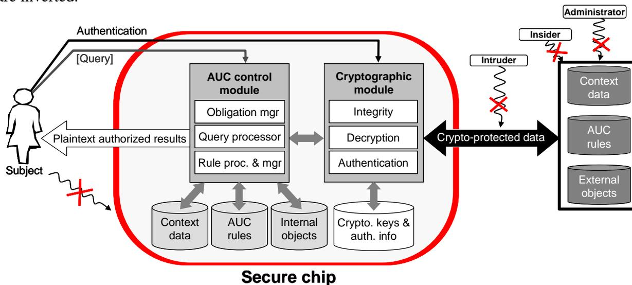
Figure 2. Functional architecture of a trusted AUC system
