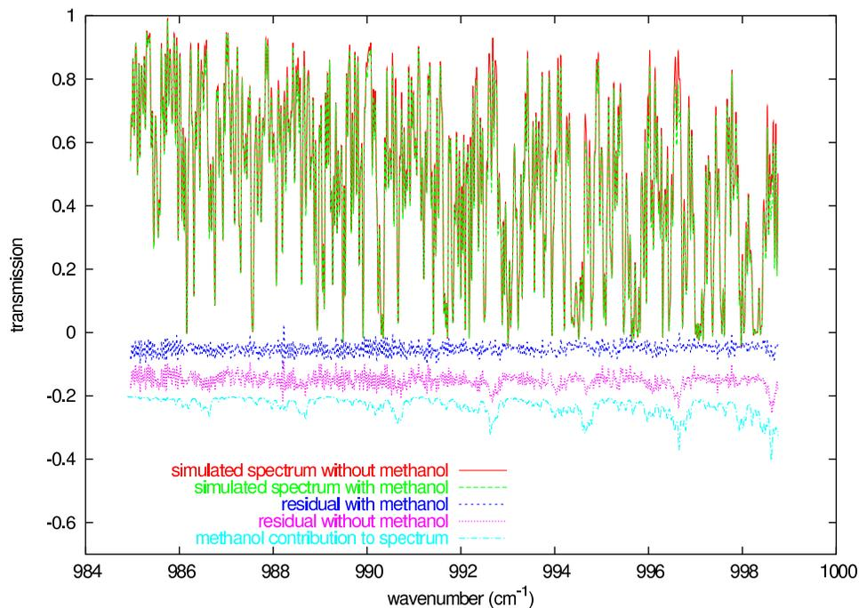
**Fig. 1.** Simulated spectra with methanol included or excluded in the calculation. The corresponding residuals (observed – calculated) and the computed contribution of  $\text{CH}_3\text{OH}$  to the spectrum using the retrieved vmr are plotted (shifted downwards for clarity).
