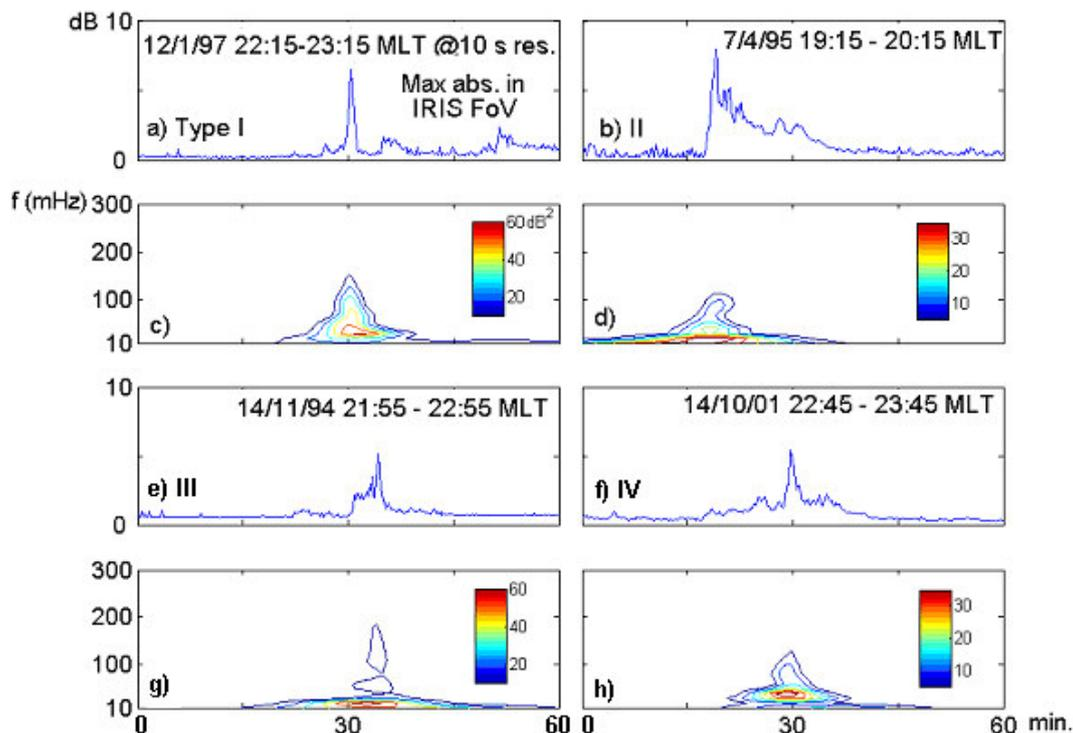
**Fig. 6.** Wavelet spectrum of 4 types of spike events. Panels (a), (b), (e) and (f) are maximum absorption in IRIS FoV in dB at 10-s resolution. Panels (c), (d), (g) and (h) are corresponding wavelet spectrum, respectively. Colorbar contours are in  $\text{dB}^2$  and the range of frequency is between 10 and 300 mHz. Data in all panels have 1-h period (x axis).
