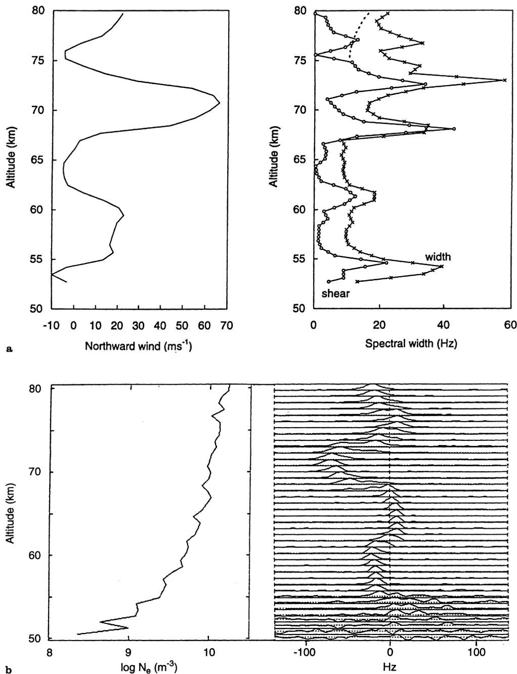
**Fig. 5.** **a** As Fig. 3, but for an antenna elevation of 45° at 1330 UT. **b.** The *right panel* shows measured VHF power spectra (arbitrary linear power scale) for the same time as part a. Each spectrum is
