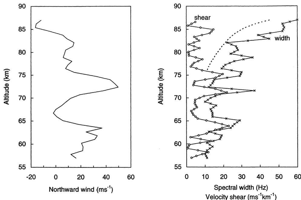
**Fig. 3.** *Left:* altitude profile of horizontal meridional wind measured with an antenna elevation angle of  $50^\circ$  at 0952 UT, 20 March 1990. The results are from analyses of 2-min integrations of the raw VHF
