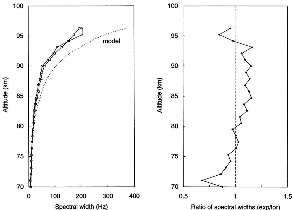
**Fig. 2.** The *left panel* shows measurements of spectral width by the EISCAT VHF radar with a vertically pointing antenna compared with model values. The profile with *open square symbols* ( $\square$ ) is from the results of fitting exponential curves to the ACFs while that with *crosses* ( $\times$ ) shows the results of fitting Lorentzian curves to the spectra.
