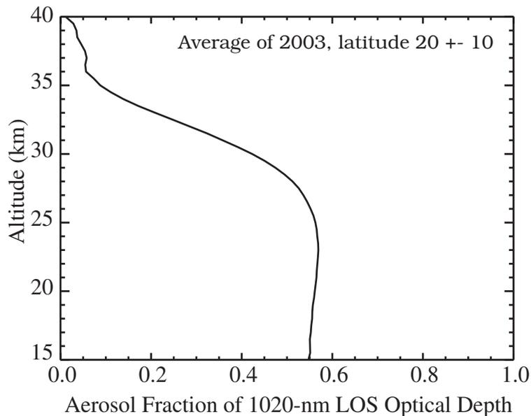
**Fig. 5.** Fraction of the measured slant path optical depth in the 1020-nm channel that is attributed to aerosol. All events between 10° N and 30° N in 2003 are included in the average shown here. Under the conditions of interest the  $\text{H}_2\text{SO}_4\text{-H}_2\text{O}$  aerosol is expected to fully evaporate at temperatures above  $\sim 238$  K, corresponding to altitudes between 35 km and 40 km.
