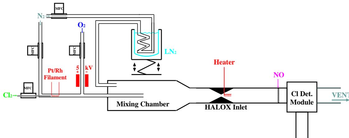
**Fig. 4.** Set up of the ClO-dimer validation/calibration system. All gas flows are regulated by mass flow controllers (MFCs). Temperatures are measured at the inlet heater, at the NO injector and directly behind the chlorine detection module. Pressure and flow velocity are also measured directly behind the detection module. A butterfly valve placed at the HALOX exhaust regulates the flow to maintain a constant pressure inside the measurement duct.
