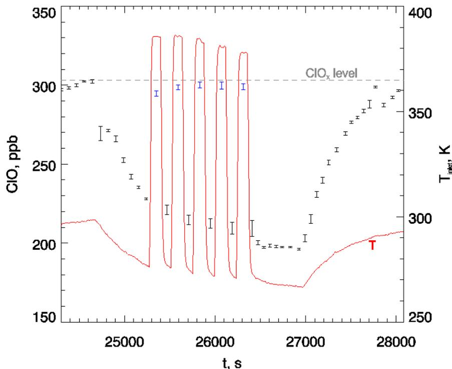
**Fig. 5.** Laboratory test ( $P_{duct}=80$  hPa) of dimer conversion efficiency of the heated inlet. Error bars represent the standard error of the mean for one minute averages (equivalent to six NO addition cycles), blue colour indicates that the temperature (red line) of the inlet heater was at the dimer dissociation temperature ( $363\text{ K} < T < 383\text{ K}$ ). The dashed line indicates the reference ClO concentration measured without cooling or heating.
