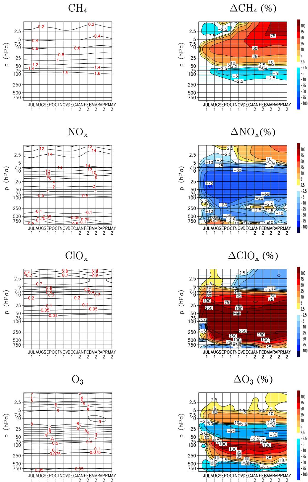
**Fig. 9.** Altitude-height cross section of the tropical averaged ( $30^\circ\text{S}$ - $30^\circ\text{N}$ ) trace gas concentrations in the control run and the simulated changes between the disturbed (YESTJUN) and the control run.
