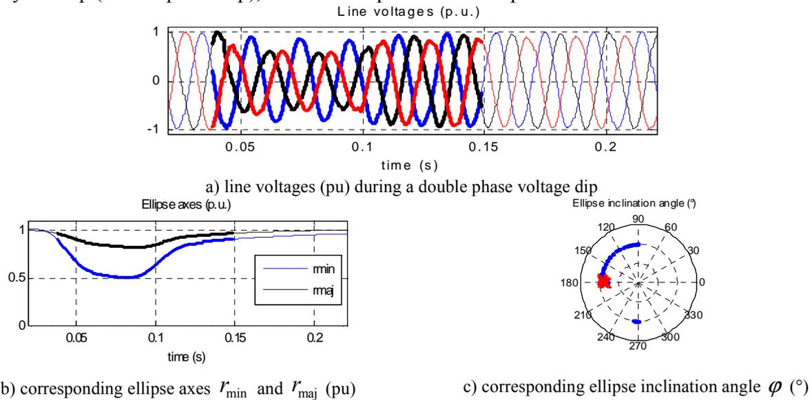
Figure 5: Monitoring of three-phase voltage dips through the space vector method
