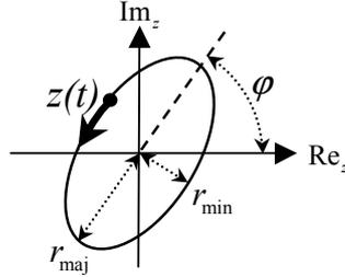
Figure 2: 2D representation of a mono-frequency complex-valued signal
