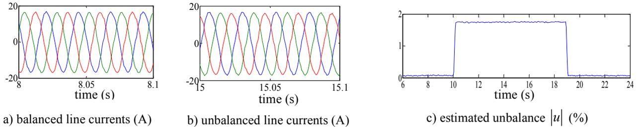
Figure 4: Monitoring of induction machine electrical unbalance through the space vector method
