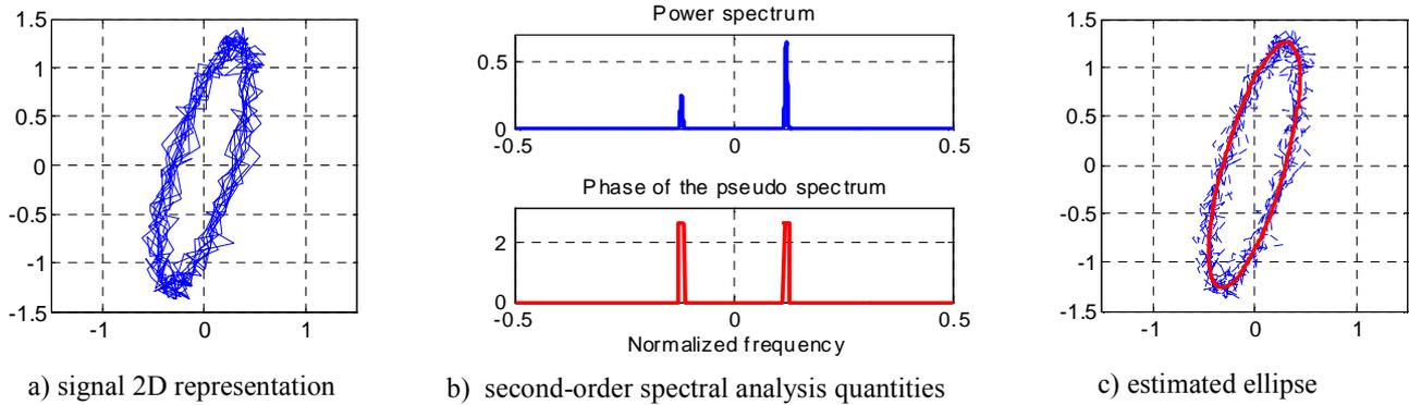
Figure 3: Second-order spectral analysis of a noisy mono-frequency complex-valued signal
