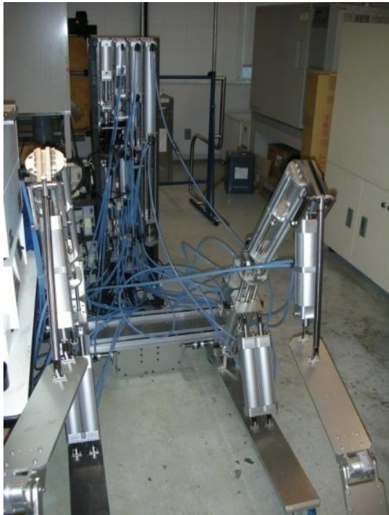
Fig. 3 : the two units are linked by the bilateral servo system. Note that short pipes are used for the moment.
