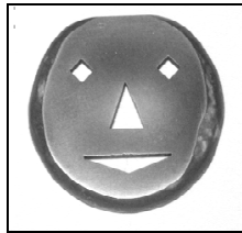
Fig.5. Disk obtained by EDM (SiC-HfB 2 , 75-25 mol%) diameter 25 mm, thickness 2,5 mm
