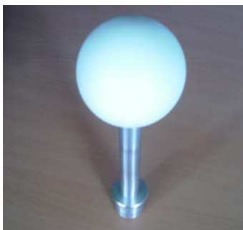
Fig. 6a: Target spheres with forced centring device
