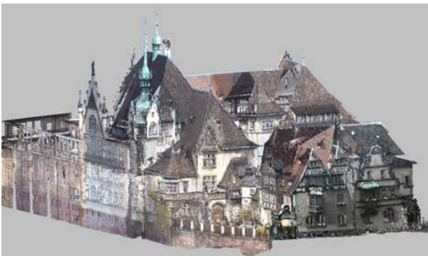
Fig. 16. Overview of the global cloud point after merging all objects of the project
