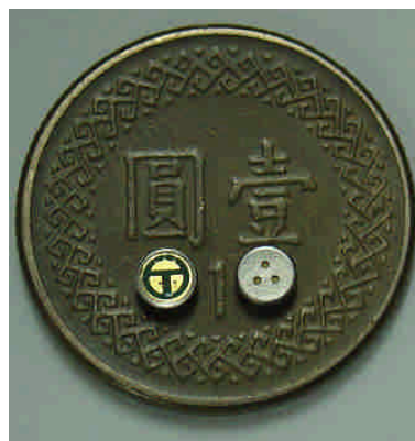
Fig. 6. A packaged condenser microphone on a coin.
