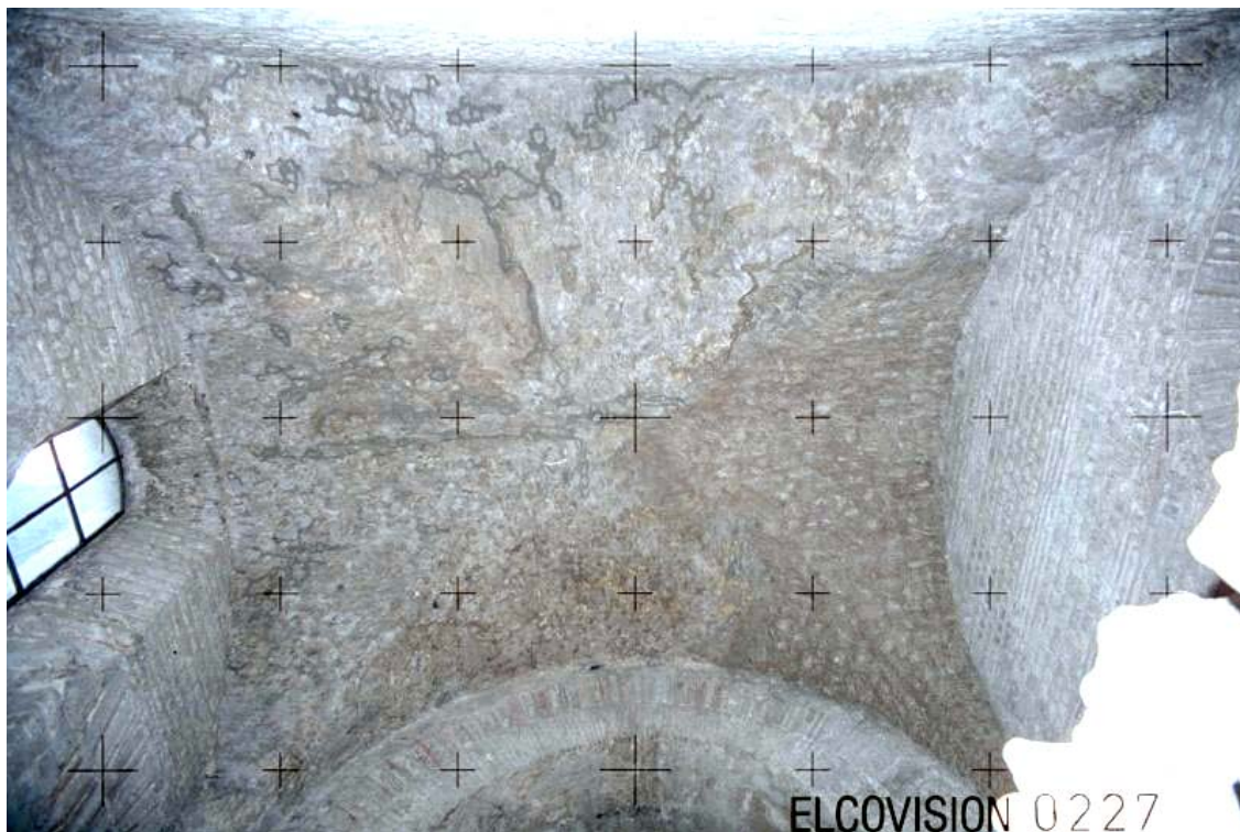
Figure 7. Shooting with a semi-metric camera 24 x 36.
