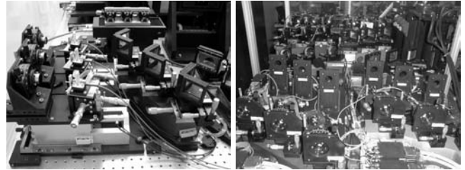
Fig. 4. Pictures of the K-spatial filter entrance. Left (picture by Y. Bresson, OCA): the three beams meet the dichroics and the parabolic off-axis mirrors before the injection through the Si birefringent single-mode fibers; Right (picture by A. Delboulbé, LAOG): the optical configuration is repeated at the exit of the fibers. Diaphragms control the beam size at the exit of the fibers and shutters select the interferometric arms.
