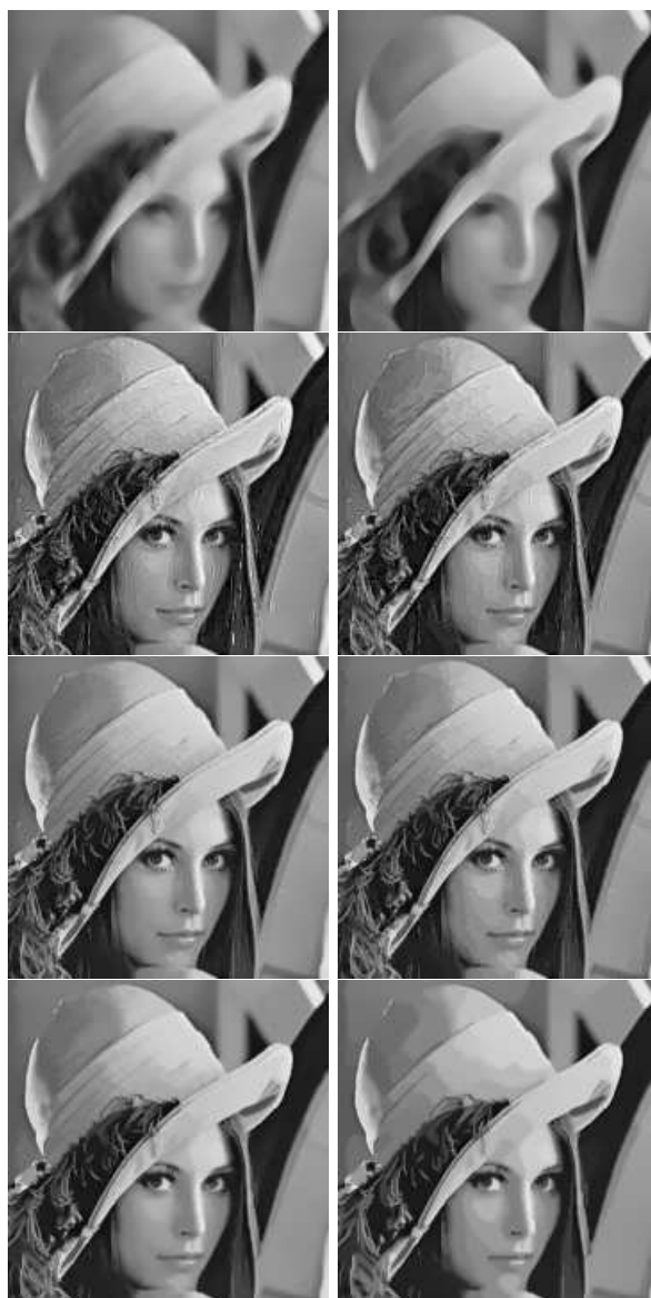
FIGURE 3.2. Comparison of linear (left images) and nonlinear (right images) diffusion schemes. From top to bottom: original image, mean curvature motion, the Perona-Malik equation, the sigma filter and the NL-means. This experiment shows first that linearized versions are more faithful for the original. This is not a surprise, since the original image features are kept in the linearized version while they are updated in the nonlinear version. The third row illustrates how much better the linearized version of the neighborhood (or sigma-, or bilateral) filter performs with respect to the non linear one. We observe the same effect in the NL-means algorithm. The iterated version produces shocks as the neighborhood filter, which are avoided by its linear counterpart. See Section 3 for more details.
