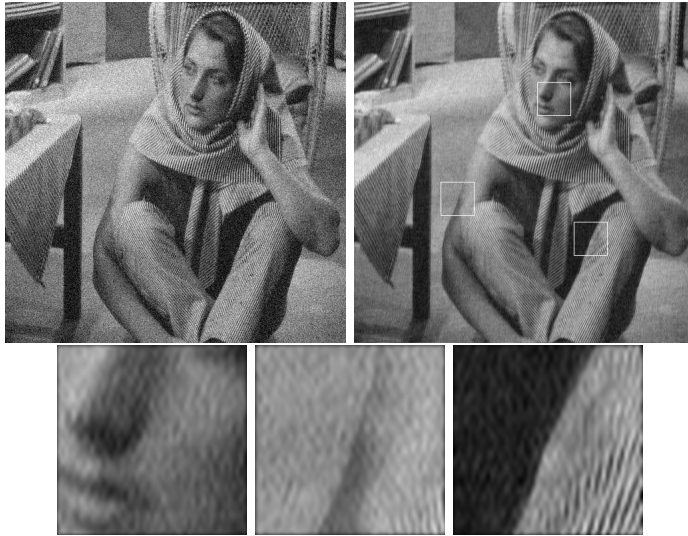
FIG. 3.1. Fourier Wiener filter experiment. Top Left: Degraded image by an additive white noise of \sigma = 15 . Top Right: Fourier Wiener filter solution. Down: Zoom on three different zones of the solution. The image is filtered as a whole and therefore a uniform texture is spread all over the image.
