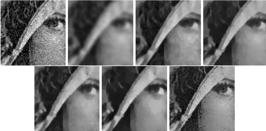
FIG. 2.2. Denoising experience on a natural image. From left to right and from top to bottom: noisy image (standard deviation 20), gaussian convolution, anisotropic filter, total variation minimization, Tadmor et al. iterated total variation, Osher et al. iterated total variation and the Yaroslavsky neighborhood filter.
