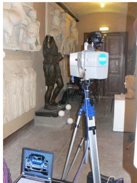
Figure 2. The TLS and the statue to digitize.
