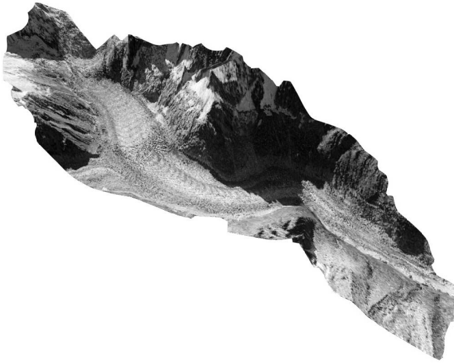
Figure 3: Mer de Glace glacier 3D-model (photos draped on the DTM) computed from the 1995 photos.
