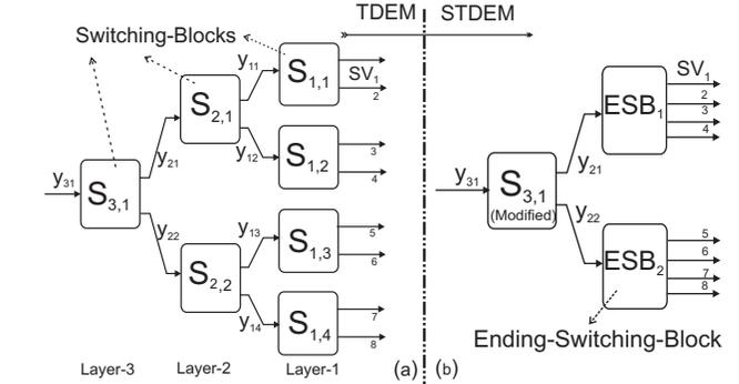
Fig. 1. Dynamic element matching algorithm: a)TDEM, b)STDEM
