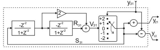
Fig. 4. Modified SB, used in all layers in STDEM but the last-one
