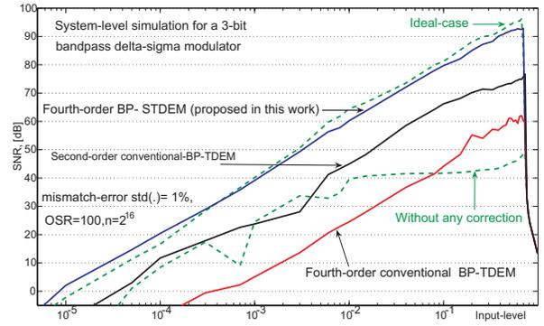
Fig. 8. Performance comparison between TDEM and STDEM algorithms
