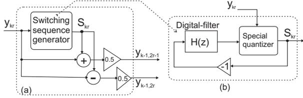
Fig. 2. a)Conventional SB's structure b)switching sequence generator
