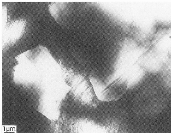
Figure 3 : TEM micrograph showing fine scale features of the microstructure present at the middle section of a 150 \mu\text{m} thick material.
