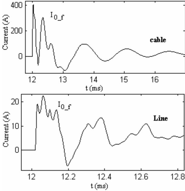
Fig. 2. The faulty feeder zero sequence currents in cables and lines of the same length and power transfer, with  $1\Omega$  fault resistance and  $90^\circ$  inception angle. The discharging components in cables are of higher amplitudes than the charging components and the frequency ratio are different in cables and in lines.
