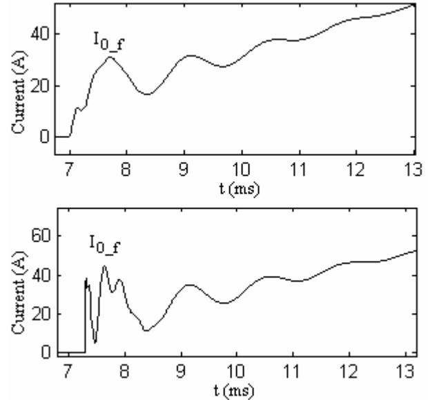
Fig. 1 Initial faulty feeder zero sequence currents in cables. The discharging currents of higher frequency are superimposed on the charging ones of lower frequency. Upper figure:  $\theta=0^\circ$ , no discharging components. Bottom:  $\theta=5^\circ$ , the discharging current's amplitude reach the level of charging components.
