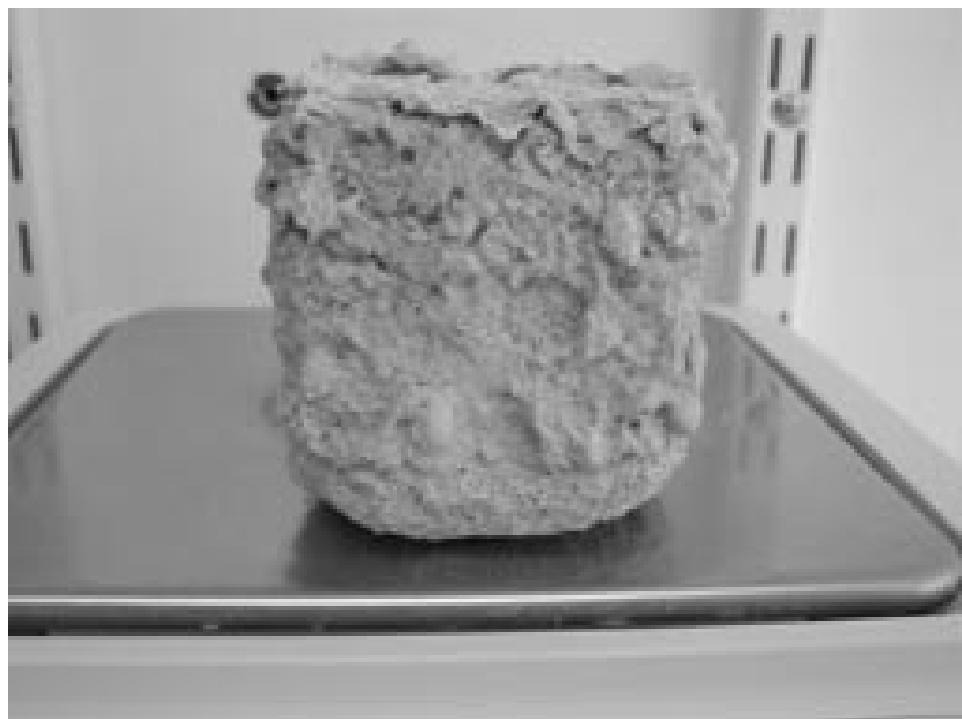
**Figure ART4-9a.** Picture of a  $7 \times 7 \times 7$  cm $^3$  non-isolated sample of FL after cycle 12.
