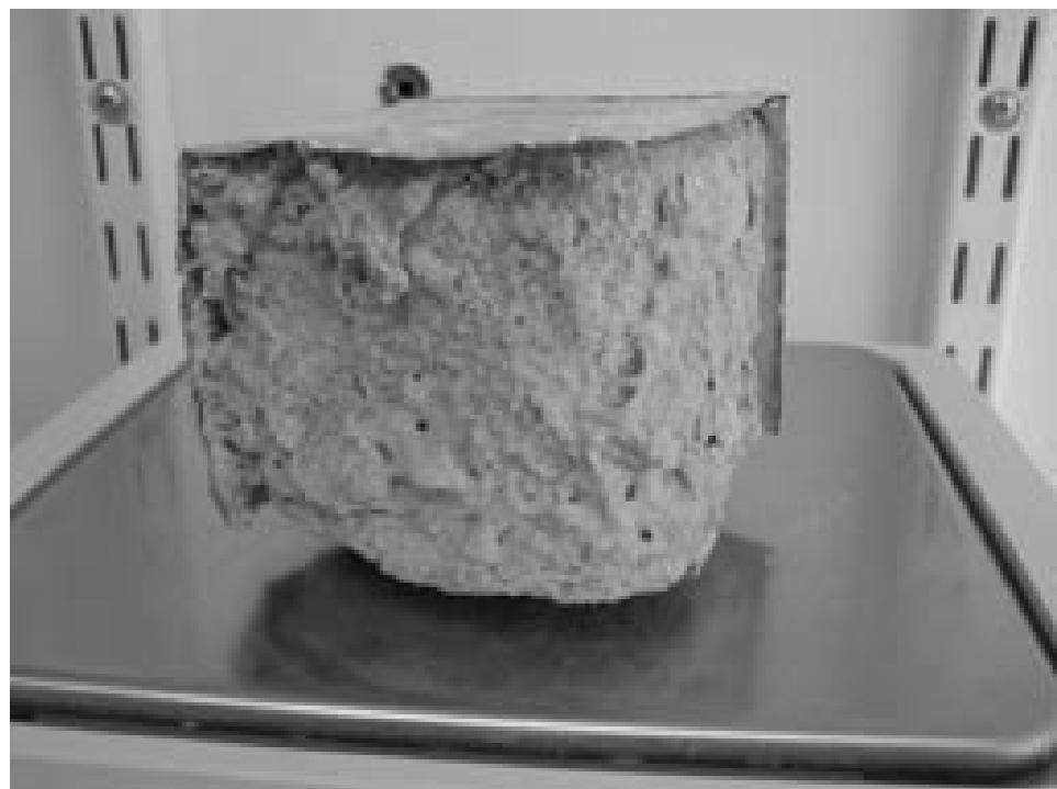
**Figure ART4-9b.** Picture of a  $7 \times 7 \times 7$  cm $^3$  sample of FL with 3 faces isolated after cycle 12.
