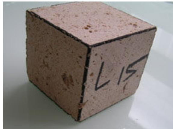
**Figure II-2.** Cube of 7cm side of the biodetritic cemented limestone LL (“liais”).
