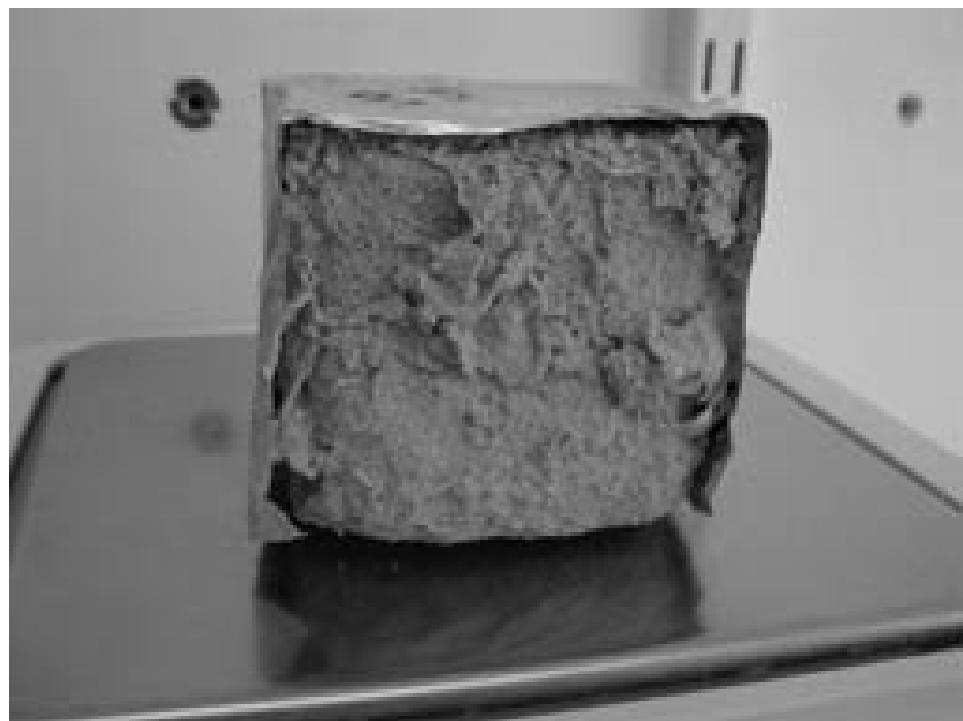
**Figure ART4-9c.** Picture of a  $7 \times 7 \times 7$  cm $^3$  sample of FL with 4 faces isolated after cycle 12.
