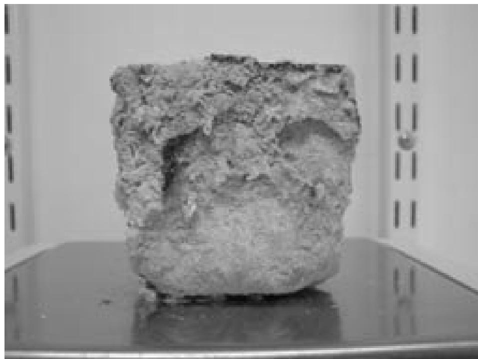
**Figure ART4-4b.** Picture of a  $7 \times 7 \times 7$  cm $^3$  sample of FL after 6 cycles of capillary imbibition & remobilisation.
