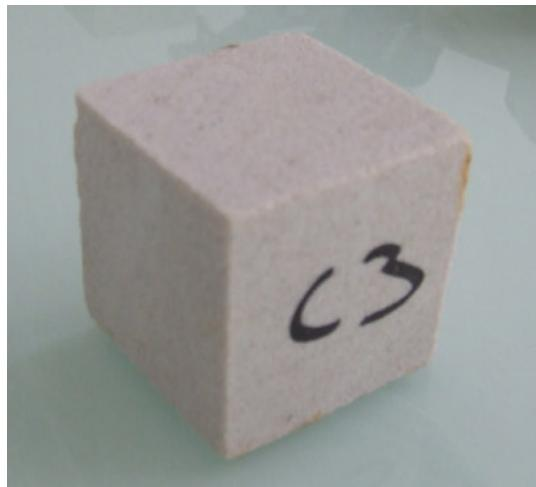
**Figure II-14.** Sample of the Chinese sandstone (CS).
