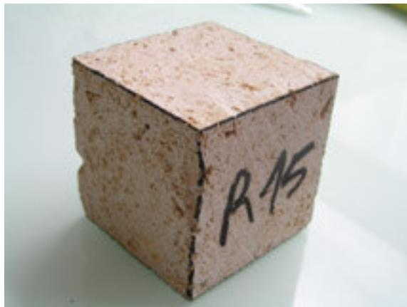
**Figure II-1.** Cube of 7cm side of the biodetritic cemented limestone RL (“roche franche”).
