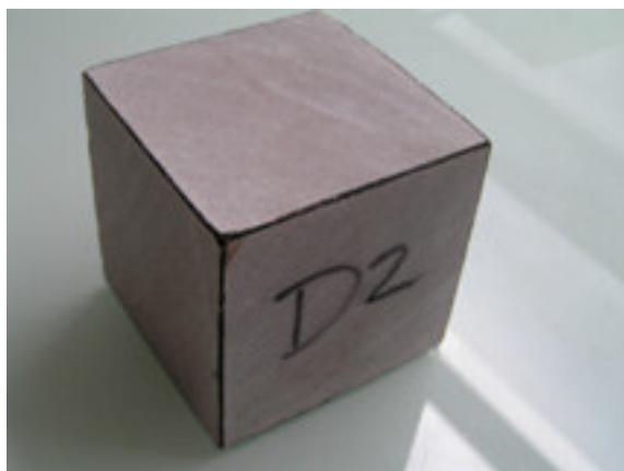
**Figure II-11.** Sample of hard Fontainebleau sandstones (HF).
