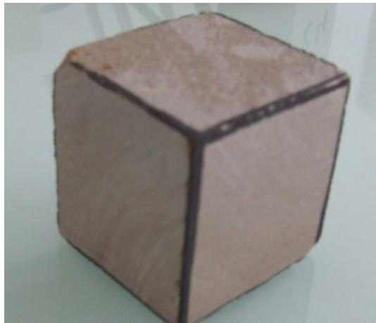
**Figure II-15.** Sample of the red Agra sandstone (MS).
