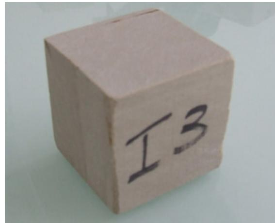
**Figure II-16.** Sample of the green Agra sandstone (VS).
