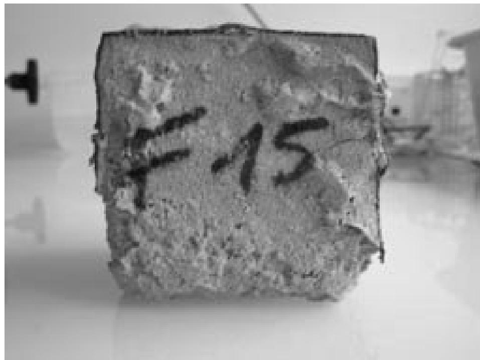
**Figure ART4-4a.** Picture of a  $7 \times 7 \times 7$  cm $^3$  sample of FL after 6 cycles of capillary imbibition.
