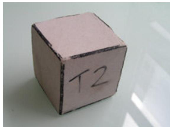
**Figure II-12.** Sample of soft Fontainebleau sandstones (SF).
