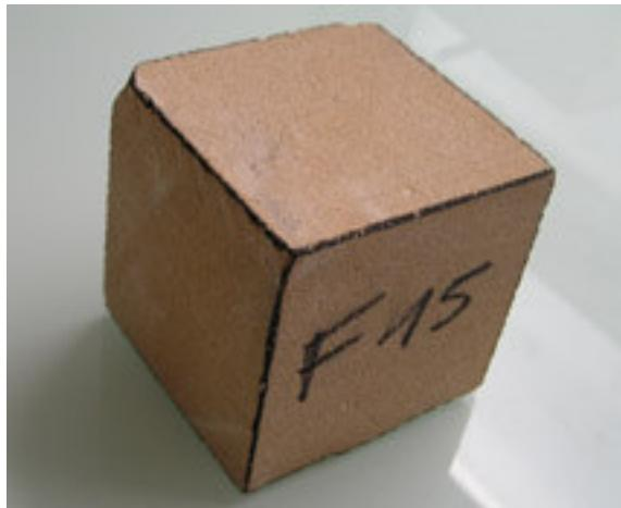
**Figure II-3.** Cube of 7cm side of the detritic limestone FL (“roche fine”).
