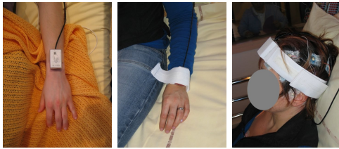
Fig. 1. Attitude sensors (AS) set on patients in an epilepsy unit. On the left, a silicon rectangular parallelepiped was first set on a wrist with adhesive tape. For patient and staff convenience, special dedicated self gripping belts were designed and set on the left wrist (middle), right wrist (not shown) and on the head (right).
