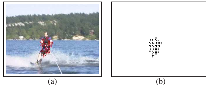
Figure 2: Observations obtained with [8] on a water skier sequence shot by a moving camera. (a) Detected moving clusters superposed on the current frame. (b) Mask of pixels characterizing the observation.
