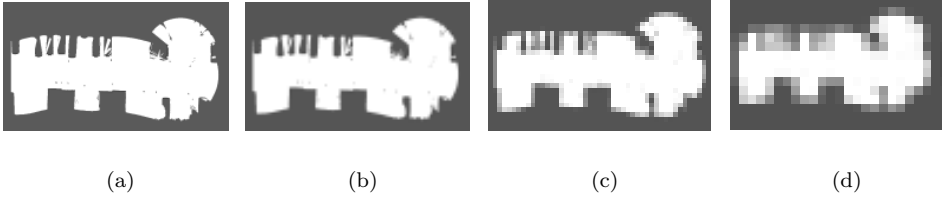
Fig. 8. Scaled view of OG provided in WavOG representation (a) scale \frac{1}{16} : 192 \times 128 pixels, s = 2 . (b) scale \frac{1}{64} : 96 \times 64 pixels, s = 3 . (c) scale \frac{1}{256} : 48 \times 32 pixels, s = 4 . (d) scale \frac{1}{1024} : 24 \times 16 pixels, s = 5 .
