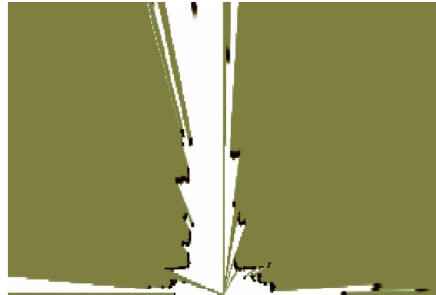
Fig. 6. Occupancy grid obtained from a laser range-finder.
