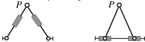
Figure 1a: A bipod PKM Figure 1b: A biglide PKM
