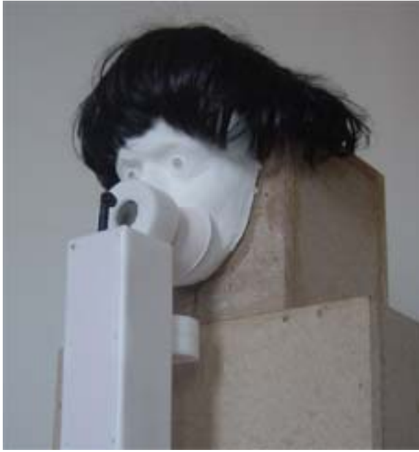
Fig 4 Artificial head loudspeaker to study acoustic distortion
