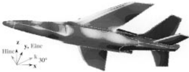
Fig. 8. Scattering of a 100 MHz plane wave by a plane considered as a perfect electric conductor. Visualization of magnetic field (in A/m).
