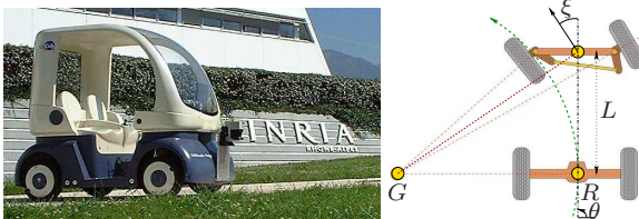
Fig. 5. The Cycab vehicle and its kinematics.
