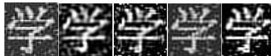
Fig. 14. Image reconstruction with M = 35 for 5% salt-and-pepper noise-contaminated binary image. From left to right are DCT and Legendre, Tchebichef, Krawtchouk ( p_1 = p_2 = 0.5 ), and Racah moments ( a = \alpha = 10 , b = 50 , and \beta = 5 ), respectively.
