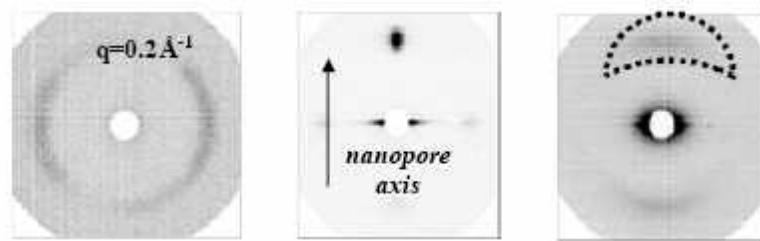
Figure 2. Small angle neutron scattering patterns of 8CB in the smectic phase. (a) bulk at 300K. (b) Confined in the channels of porous alumina at 300K. (c) Confined in the channels of porous silicon at 290 K.
