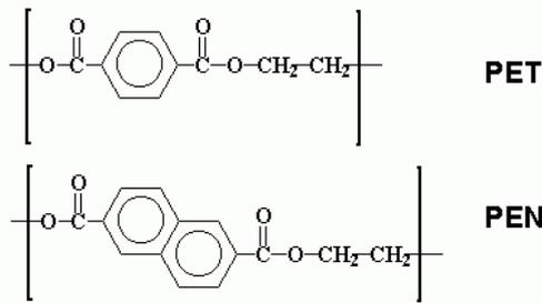
Figure 1 Molecular structures of polyethylene terephthalate & polyethylene naphthalate.
