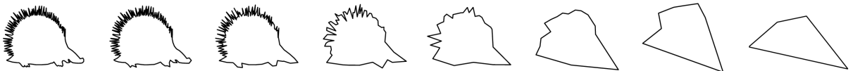
Figure 6: Multiresolution analysis of quadratic uniform B-spline curve. From left to right the initial curve with 512 control points, and the control polygons of its seven coarse approximations (each having 2^i , i = 8, \dots, 2 control points) are shown.
