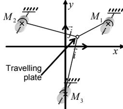
fig. 2 – Geometry of a typical parallel wire-driven mechanism
