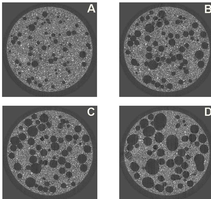
**Figure 4** Evolution of pore structure at the same level in the stack as in figure 3 of a cellulose ether modified cement paste (water to cement ratio equal to 0.5) at 16 min (a), 26 min (b), 35 min (c) and 50 min (d)
