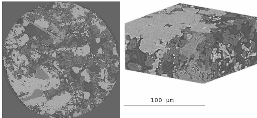
**Figure 1** 2D slice (sample diameter:  $560\ \mu\text{m}$ ) and 3D reconstruction of quarry tuffeau (limestone originating from the Loire valley, France) grey levels allow to distinguish the different components: grey light: calcite, dark grey: silica, black: porosity.
