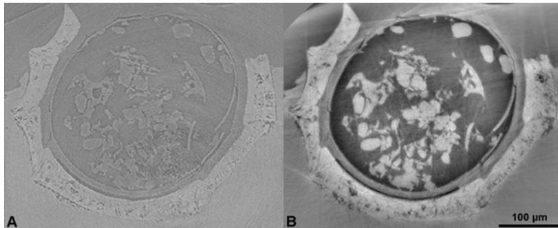
**Figure 2:** a) Absorption reconstructed slice of a charophyte (linear attenuation coefficient map) b) Same slice in holotomography (density map) (in collaboration with S. Zabler and M. Feist, Institut des Sciences de l'évolution de Montpellier, France)
