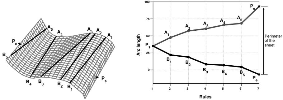
Figure 3: (left) The generated mesh with the control points  $(A_i, B_i)$ . (right) Arc lengths  $s_A$  and  $s_B$  of the control points with the interpolating functions  $f_A$  and  $f_B$ .
