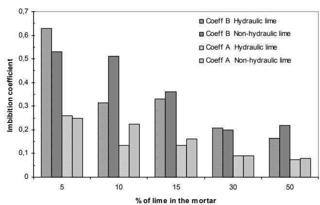
Figure 9: Imbibition coefficients for the different mortar
