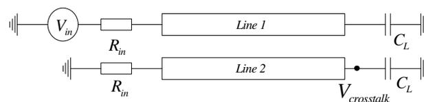
Fig. 1: Coupled-line model.
